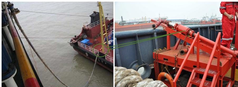
Figure 4. Quick release device and installation diagram.
