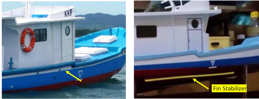
Figure 19. Fin Stabilizer addition to fishing vessel.
